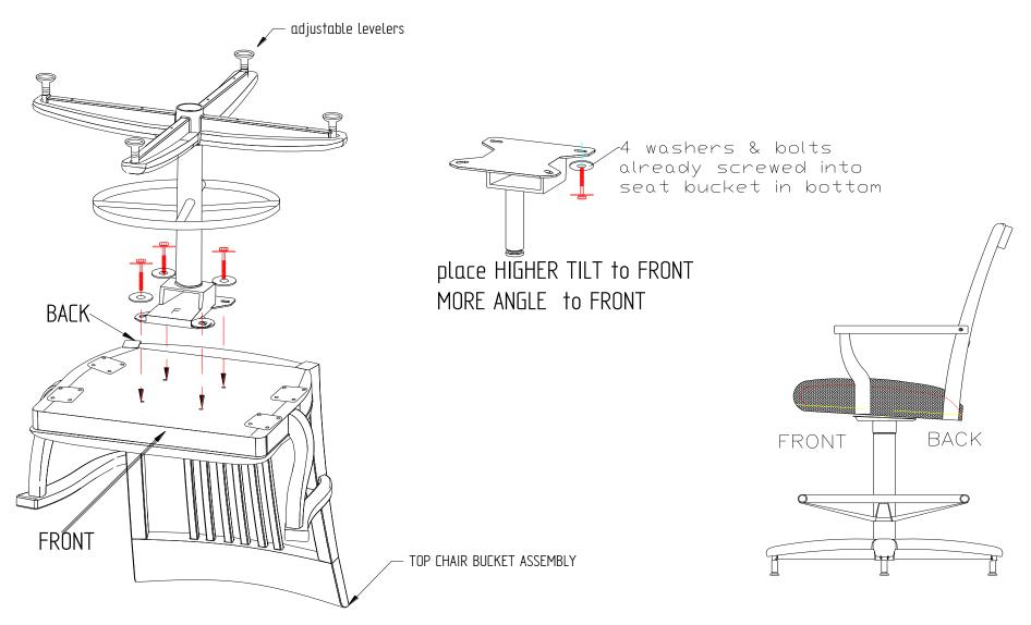
PRE-CAUTION: EVERY 6 MONTHS- RETIGHTEN THE 4 BOLTS IN THE MOUNTING PLATE. USAGE CAN MAKE SCREWS WORK LOOSE OVER TIME.
